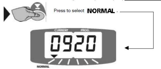
The left hand section shows the current number of wraps and the right hand section shows the target number.
