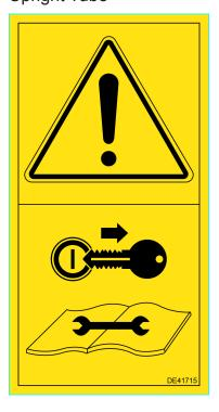
Remove key from power unit before attempting any maintenance on this machine. Item 6 on *pg. 1-3*Part No: DE41714 - Inside Face of 3 Point Hitch Upright Tube
